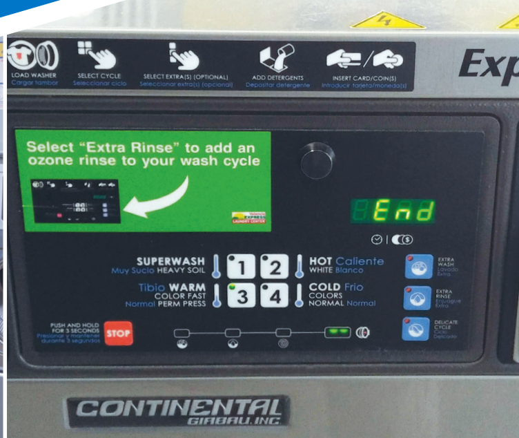
The Continental ExpressWash Washers feature the ProfitPlus Control, which offers customers four standard cycles and the option to add an extra wash, rinse or spin. If customers want to, they can choose to add an extra rinse, which is ozonated, in order to sanitize their laundry.
