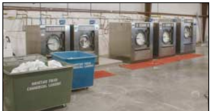
Mountain Fresh's growing business now features a 130-, two 55- and two 90-pound capacity Pro-Series washer-extractors.
